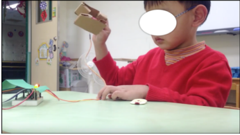
Figure 4: The first prototype. When pinching the clip harder, more LED light bulb will glow.
